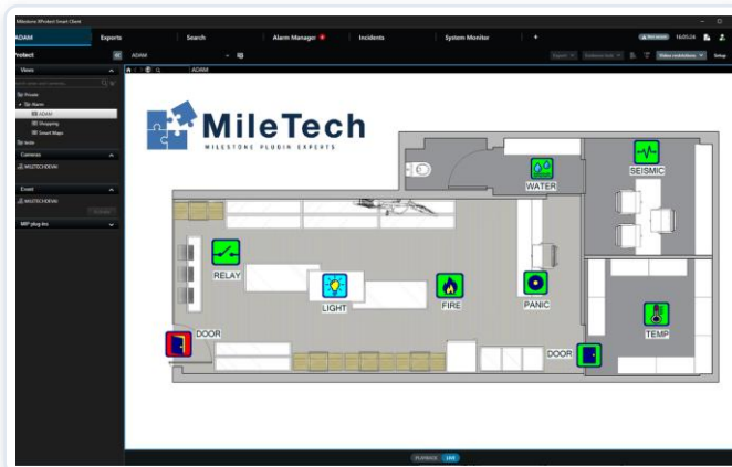
Door left open triggers an alarm on the Smart Client map
